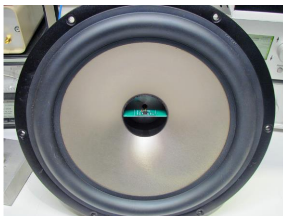
Figure 6: MFB-Sensor PCB glued into the voice coil of a loudspeaker.
