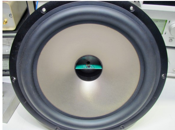
Figure 6: MFB-Sensor PCB glued into the voice coil of a loudspeaker.
