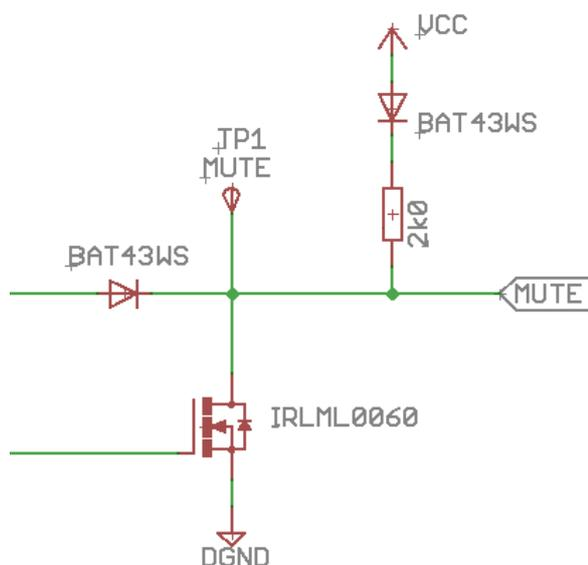
**Figure 14: MUTE Input/Output Interface (Standby identical if populated)**
