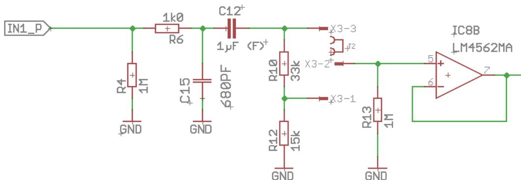
Figure 20: One Channel Audio Input Interface
