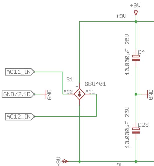
Figure 12: AC Input Circuit Diagram
