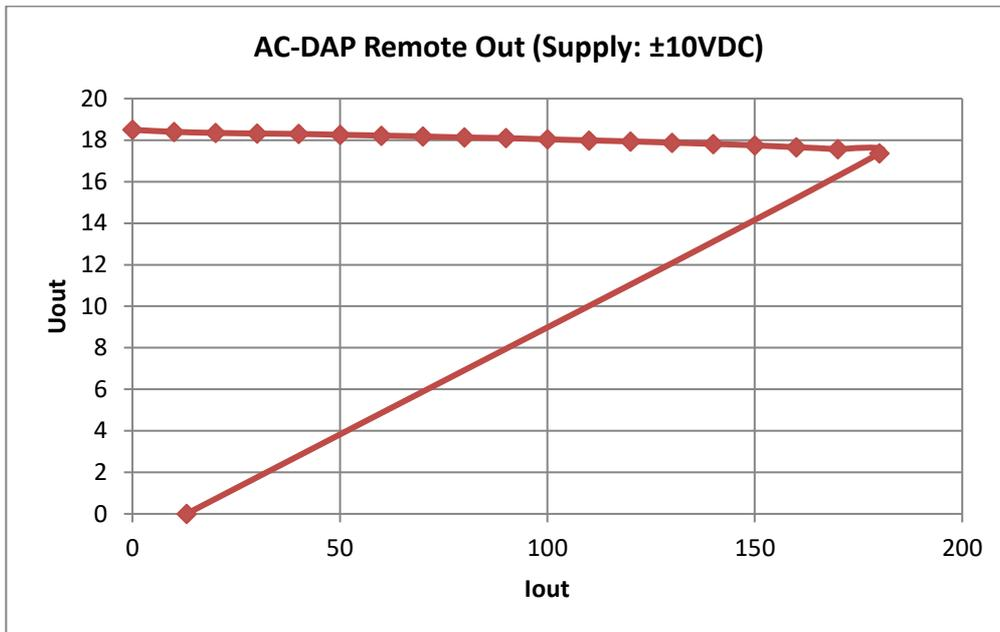
Figure 16: Remote Output driver capability and over current protection (V2/MF-R010)
