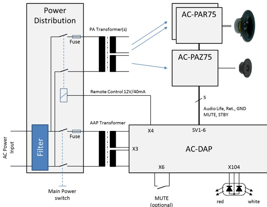
Figure 18: Recommended power distribution and control configuration
