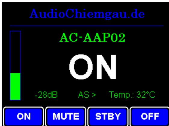
Figure 6: 3.2" Color Display with four touch buttons
