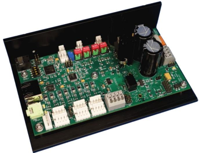
Figure 1: Digital Audio Processor AC-DAP for two-, three-, or four-way speaker systems with or without Sub-Woofer
