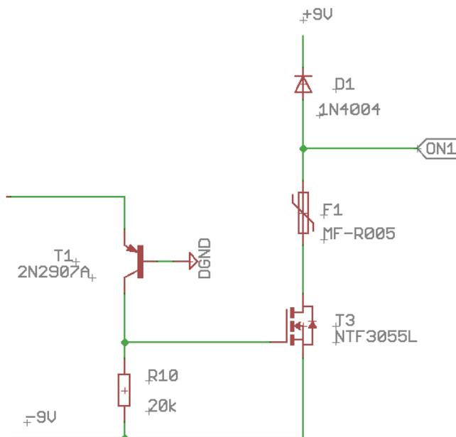
Figure 15: Relay driver stage for 2-channel ON/OFF remote control <sup>12)</sup>
