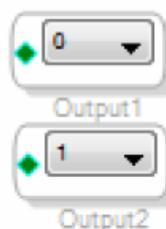
6. To connect each Input1 channel to the corresponding output block, click and drag a line representing a wire between the blue pin of the Input1 block and the green pin of the corresponding output block (see Figure). Input1 Channel 0 connects to Output1 Channel 0 and Input1 Channel 1
