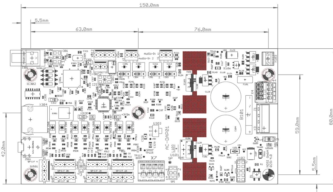
Figure 10: Layout of the PCB, top view and populated as AC-DAP (V4)
