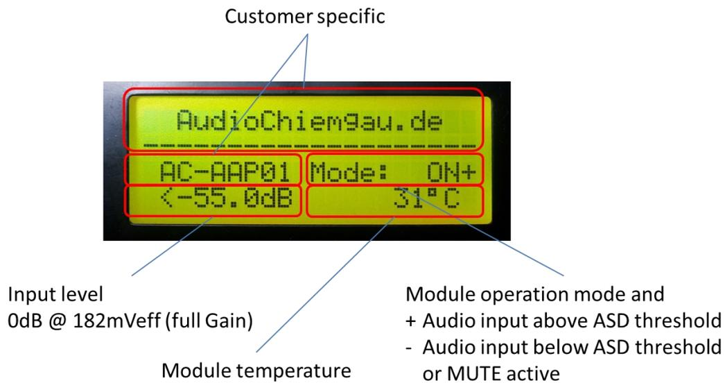
**Figure 7: Example for Tiny Display**
