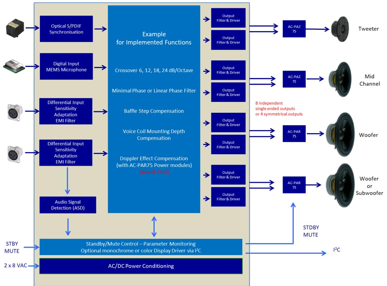
Figure 3: Examples of implementable functions
