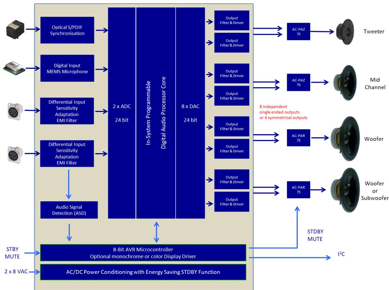
Figure 2: Block Diagram of the Digital Audio Processor AC-DAP 1)
