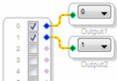
The default register settings in SigmaStudio are configured to match the AC-DAP board hardware, including the signal routing between the ADAU1452 and the AD1938 codec. When these steps are complete, the basic signal flow is complete and the stereo analog input source passes directly through the SigmaDSP and connects to the stereo analog output.
