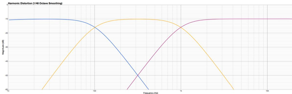
Figure 5: Frequency response of the example filter implementation
