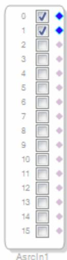
Because the left and right signals of the S/PDIF receiver pass through the ASRC0, the input to the DSP program is the Asrcin1 block in SigmaStudio. The naming convention for the input and output blocks is such that all blocks in SigmaStudio are named from the perspective of the DSP core. Therefore, the Asrcin1 block in SigmaStudio represents the input to the DSP from the ASRC outputs.
