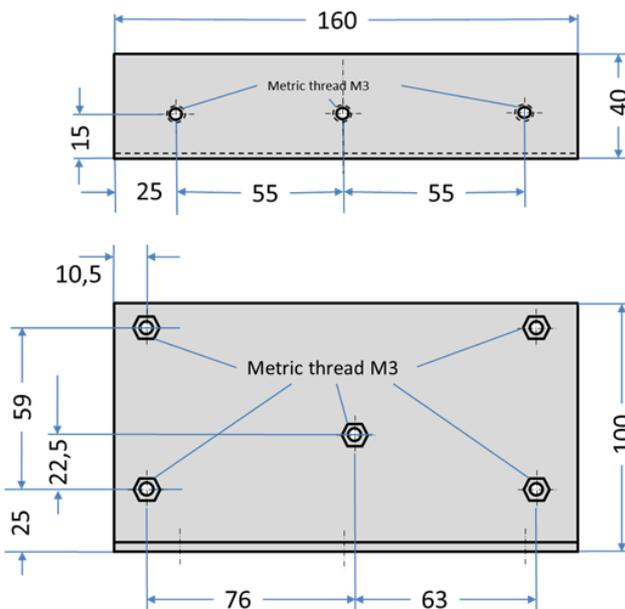
Figure 11: Flange for vertical mounting of the module
