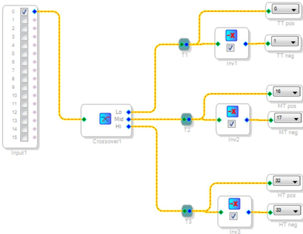
Figure 4: Example of programming the AC-DAP through the SigmaStudio® Graphical User Interface
