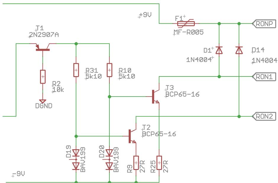
Figure 17: Relay driver stage for 2-channel ON/OFF remote control (constant current driver) <sup>13)</sup>
