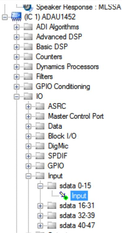
and then dragging it into the empty project space. The Input1 block, which represents an input channel, then appears as shown in the Figure. By default, Channel 0 and Channel 1 are selected and this configuration matches the analog audio source hardware connections. Therefore, no modifications are needed.
