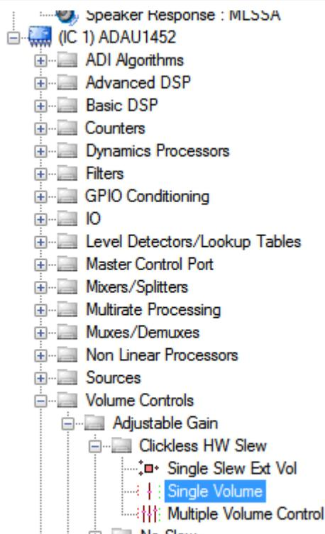
2. By default, the Single1 block has one input and one output, meaning it is a single channel. To add another channel, right-click the empty white space of the Single1 block and from the drop-down menu that appears, select the Grow Algorithm > 1. Gain (HW slew) > 1 option (see Figure).
