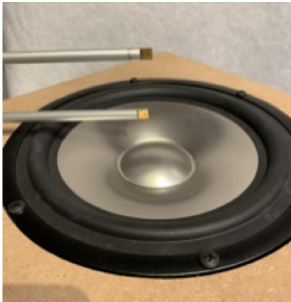
Figure 1: Two MEMS microphones located 5 cm and 10 cm from membrane
