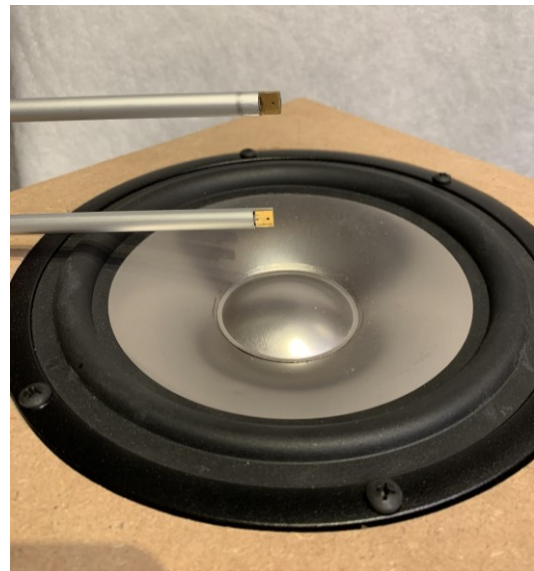
Location of the microphones on an axis perpendicular to the membrane
