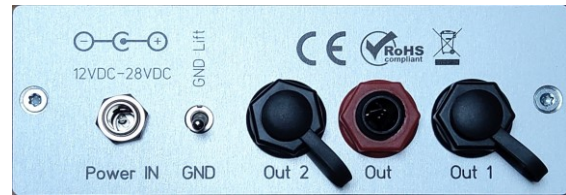
Connectors on the rear side of the control unit
