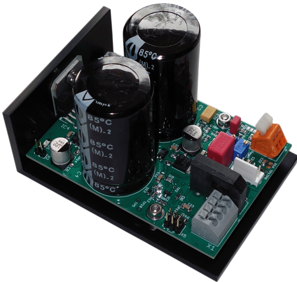
Figure 3 : AC PAR75 Integrated amplifier module comprising the complete acceleration control circuitry. On the right side: Sensor PCB mounted inside the voice coil with flex lead-out.
